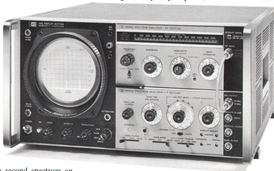
Fig. 1. A new plug-in RF section makes this a 0.5-to-1250-MHz spectrum analyzer—or frequency-domain oscilloscope, if you prefer. It has absolute amplitude calibration, automatic phase lock, and simple controls. Its frequency response is flat within \pm 1 dB from 1 to 1000 MHz. It has a 60 dB spurious free display range, -120 dBm maximum sensitivity, and scan widths from 20 kHz to 1250 MHz. Variable-persistence and large-screen displays are optional.
